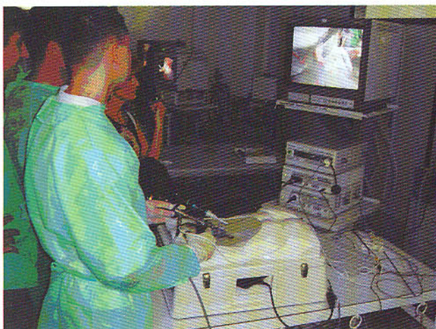
Figure 4. Practice with endoscopic trainer - true operation conditions are simulated (Split, 2003)
